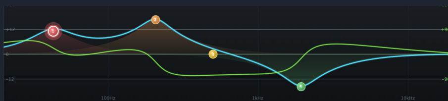
The EQ graph showing magnitude response (cyan) and phase response (lime green)
