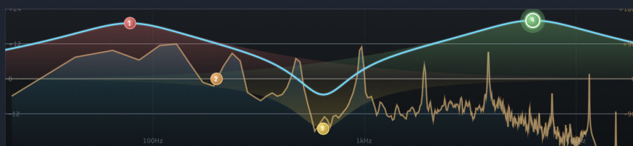
Real-time spectrum analyzer with EQ curve overlay and draggable band nodes
