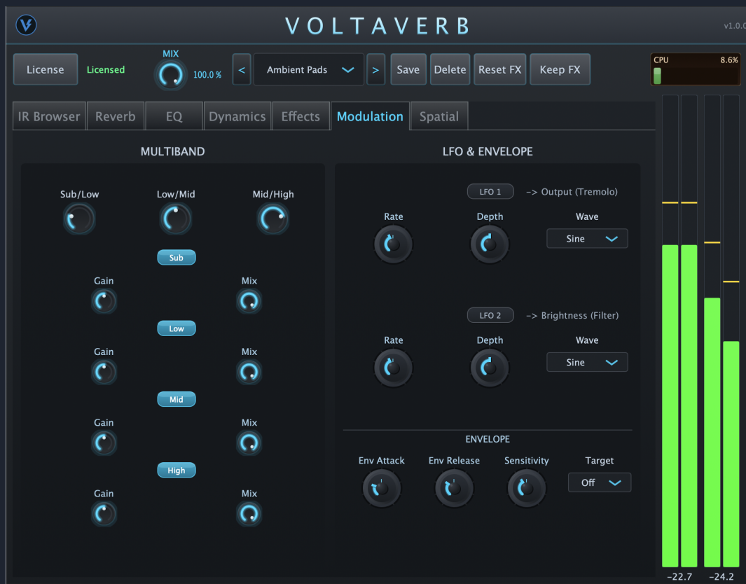
The Modulation panel with Multiband, LFOs, and Envelope Follower
