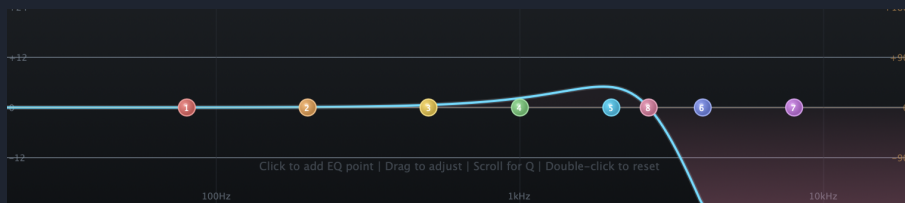
High Cut (Low Pass) — Remove frequencies above the cutoff point
